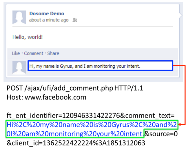
Fig. 2. An example WYSIWYS applicable operation: Facebook comment. After adding a comment and pressing the ENTER key, the application generates network traffic going to www.facebook.com/ajax/ufi/add-comment.php . There is a direct mapping of user-intended content between on-screen text and outgoing traffic.
