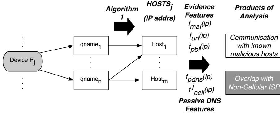
**Figure 3: Determining the communication patterns for each mobile device ( $R_j$ ). Each qname requested by  $R_j$  is converted into an IP address via Algorithm 1. This list of IP addresses ( $HOSTS_j$ ) is then processed for Passive DNS Features (PF) to determine overlap with traffic from our non-cellular ISP and for Evidence Features (EF) to determine the presence of communications with known malicious domains.**
