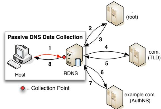
Figure 1: Example of the domain resolution process.
